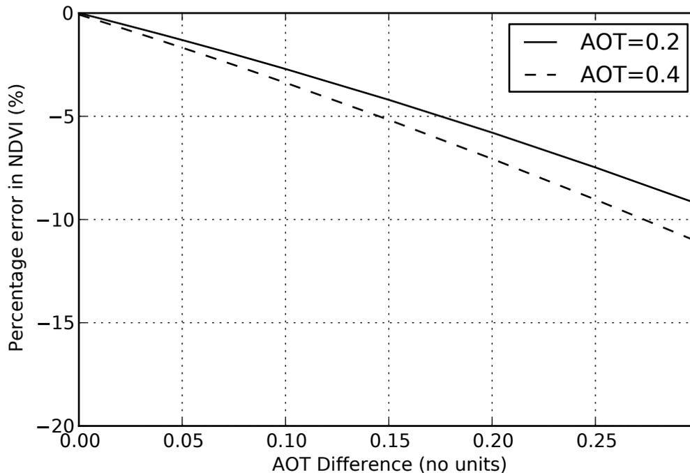
Figure 8. Sensitivity analysis showing percentage change in NDVI caused by correcting a standard green vegetation spectrum with an erroneous AOT value, for two standard AOT values (0.2, corresponding to a visibility of around 20km; and 0.4, corresponding to a visibility of around 10km). The x-axis shows the difference between the true AOT and the AOT used for correcting, and the y-axis shows the resulting error.
