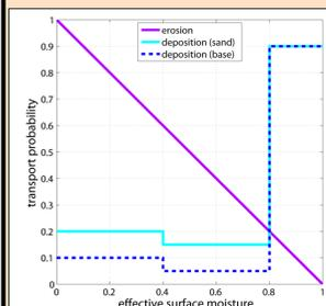
Fig. 3.1 Sediment erosion and deposition probabilities based on effective surface moisture and sediment presence.
