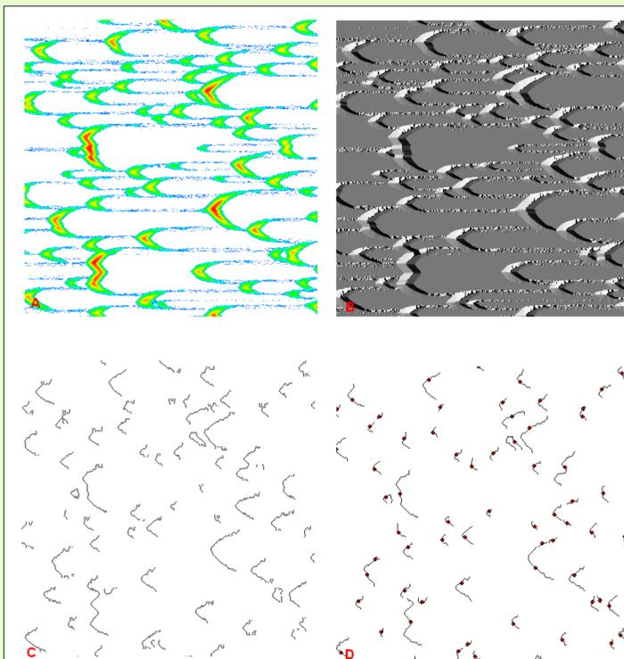
Fig. 2.1 A. example DEM, B. aspect image, C. binary crest image, D. GIS crest extraction and point insertion
