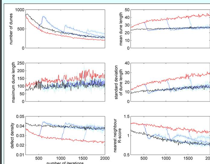
Fig. 4.1 Metric trends for  $1000 \times 1000$  grid under dry (red line) or moist (black line) conditions. Blue lines indicate trends when surface moisture influences are applied part way through a simulation. Shaded area indicates twice standard deviation for behaviour of ten simulations.
