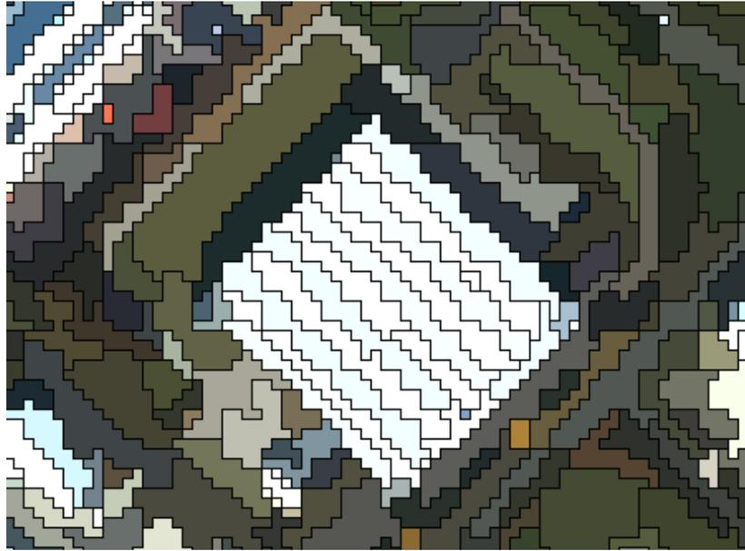
Figure 23 - Subset of Risley image showing oversegmentation of a building roof, with each sawtooth segment represented in a separate image object
